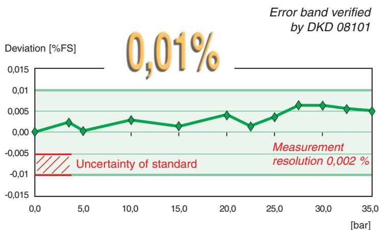
In operation, the μP attributes the exact pressure value to a set of pressure and temperature signals. By this method, called mathematical modelling, the error band is typically narrowed down by a factor of 100.
